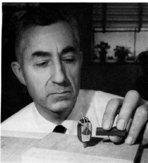
Figure 8.3 A light-commutated motor
